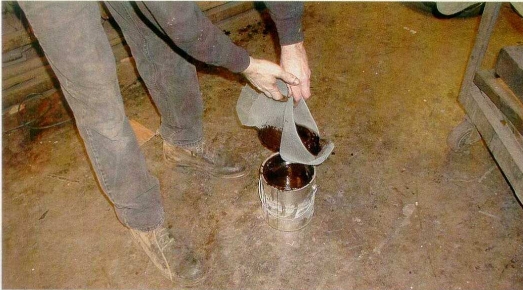
Figure 4: To be sure there aren't any dried lumps in the filler that could scratch the wood in the removal process, I strain the filler through a screen.
