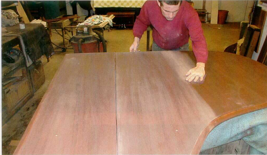
After two days of drying, I go over the filler with a final pass of maroon Scotch-Brite to make sure the wood is clean: Any streaks of filler that remain could show through the finish!
