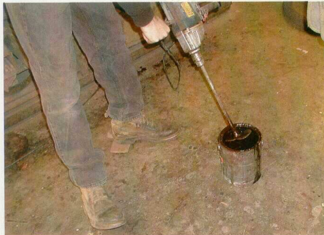
Figure 3: After I’ve added the colorant and thinner to the paste wood filler, I stir the mixture with a mixing rod on my drill.
