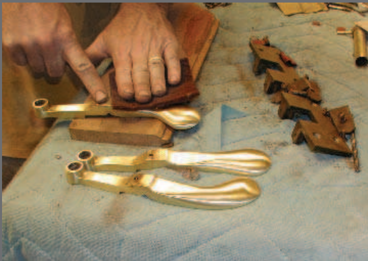
Photos 11 (LEFT) & 12 (RIGHT) – Pedals should be cleaned and sprayed with extra lacquer.
