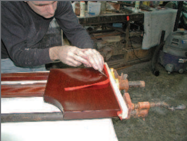
Photo 7 – Trimming excess cloth.
