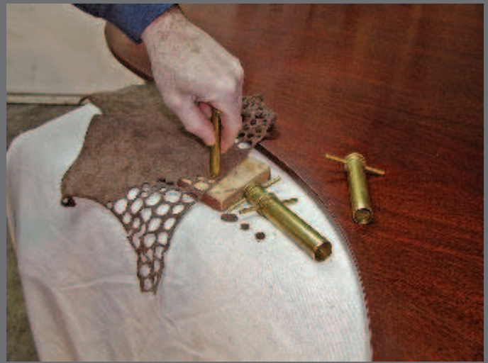
Photo 16 – Using brass circle cutters to cut two pieces of leather: one slightly larger than the hole and one slightly smaller.
