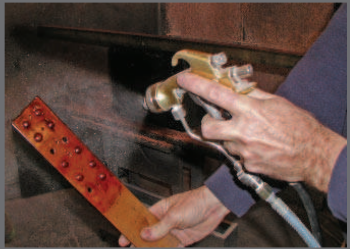
Photo 22 – Mount the buttons on a block of wood to spray the lacquer.
