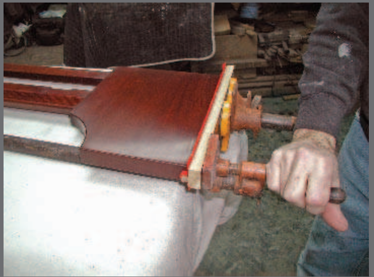
Photo 6 – After gluing the cloth, hold cauls in place with clamps.
