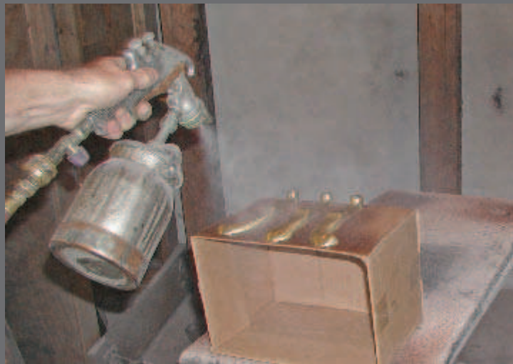
Photos 11 (LEFT) & 12 (RIGHT) – Pedals should be cleaned and sprayed with extra lacquer.
