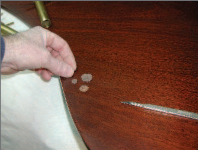
Photo 17 – The leather is cut and ready to be glued into place.
