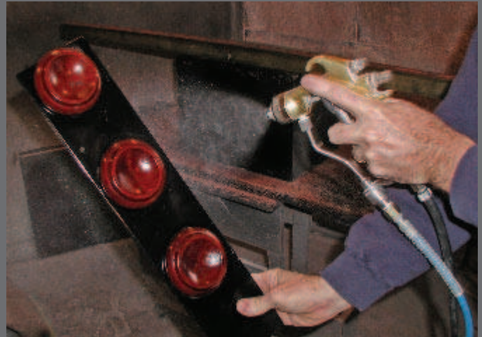
Photo 24 – The finish on the caster cups can be applied to match the piano's finish.
