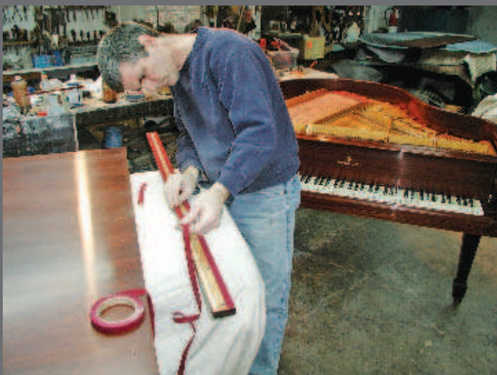
Photo 9 – Felting the lid support board.
