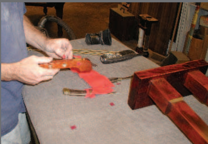
Photos 13 (LEFT) & 14 (RIGHT) – The pedal rod guide is rebushed.
