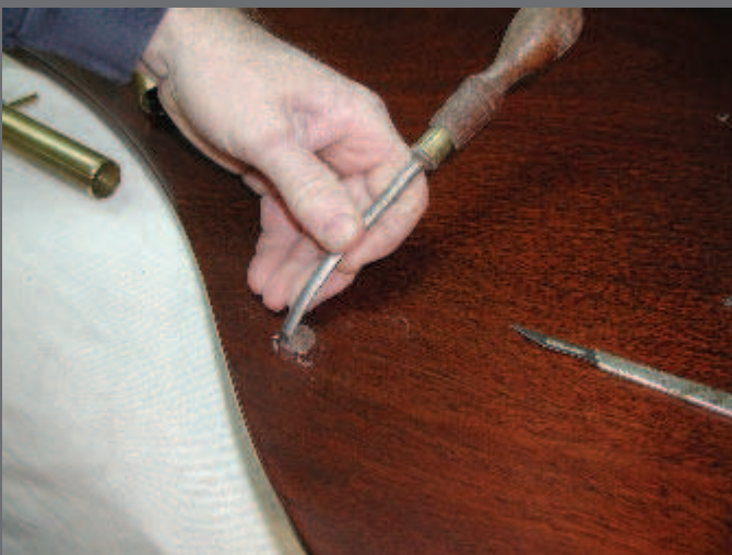
Photo 19 – With a carving gouge, tuck the button into position.
