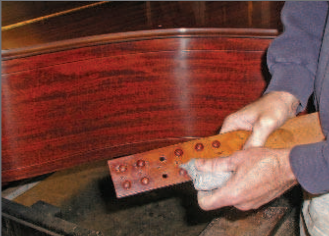
Photo 23 – Once finished, rub the buttons to match the final sheen of the lid.
