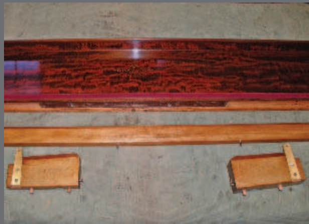
Photo 25 – The reverse sides of case parts need a coat of clear lacquer to keep out moisture.
