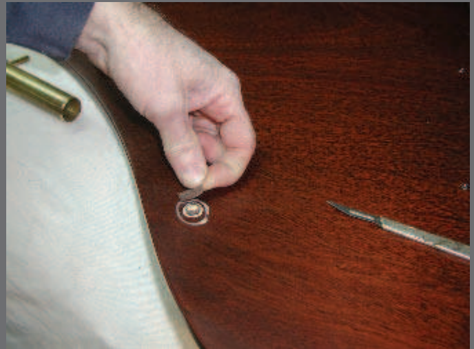
Photo 18 – Gluing the leather.
