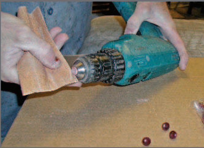
Photo 21 – Chuck wooden buttons for the lid in a hand drill, sand with 120 grit paper and then apply dye.
